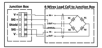
The following table displays the equivalence between load cell terminals-colors and junction box terminals.
