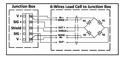
The following table shows the equivalence between load cell terminals-colors and junction box terminals.
